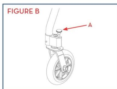
2. To unfold the Nimbo, face the open end, press the push pins, tilt the walker so that it rests only on its rear feet and push the front feet towards the rear feet.
